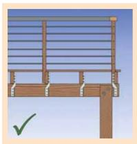
An example of floor joist spanning over supporting beams and the balustrade supports being connected directly to the supporting structure. The tension of the balustrade wire is tight.
