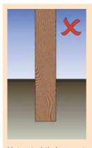
Untreated timber posts placed directly into the ground or cast directly into concrete footings are more susceptible to insect attack and rot.
