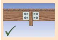
Floor joists that are fixed in between beams require more visual inspections and maintenance. Look for thick steel plates with at least two bolts in each piece of timber or properly fixed manufactured hanger brackets.
