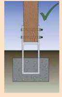
Galvanised metal brackets or stirrups which are cast into concrete footings can stop wet rot from occurring around the base of timber posts. With adequate clearance from the ground, the stirrups can be useful as a termite barrier.
