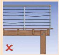
An example of floor joists fixed in between beams and the balustrade supports being connected directly to the decking. The tension of the balustrade wire is too loose.
