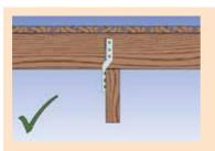
Floor joists that rest on top of beams (also called bearers) are inherently safer because the transfer of decking loads to the bearers does not depend on the fixings.
